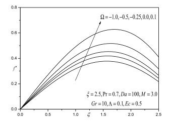
Figure 16: Effect of  $\Omega$  on the Skin friction coefficient results
