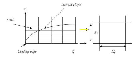
Figure 2: Grid meshing and a "Keller Box" computational cell
