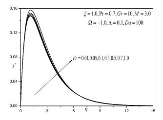
Figure 11: Effect of the Ec on the velocity profiles
