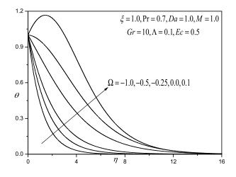
Figure 10: Effect of the  $\Omega$  on the temperature profiles.
