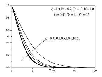
Figure 5: Effect of the  $\Lambda$  on the temperature profiles
