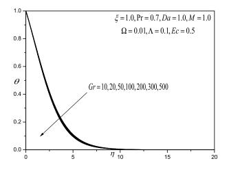
Figure 8: Effect of the Gr on the temperature profiles
