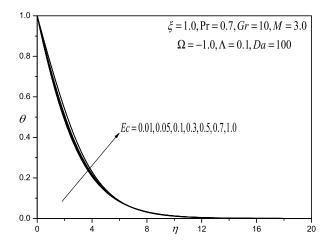
Figure 12: Effect of the Ec on the temperature profiles
