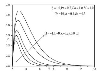
Figure 9: Effect of the  $\Omega$  on the velocity profiles.
