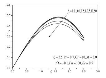
Figure 15: Effect of  $\Lambda$  on the Skin friction coefficient results.
