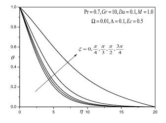
Figure 14: Effect of the  $\xi$  on the temperature profiles
