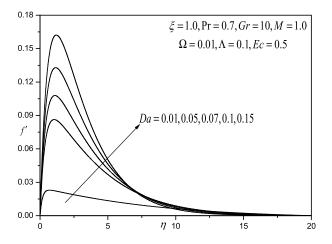
Figure 6: Effect of the Da on the velocity profiles
