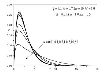
Figure 4: Effect of the  $\Lambda$  on the velocity profiles
