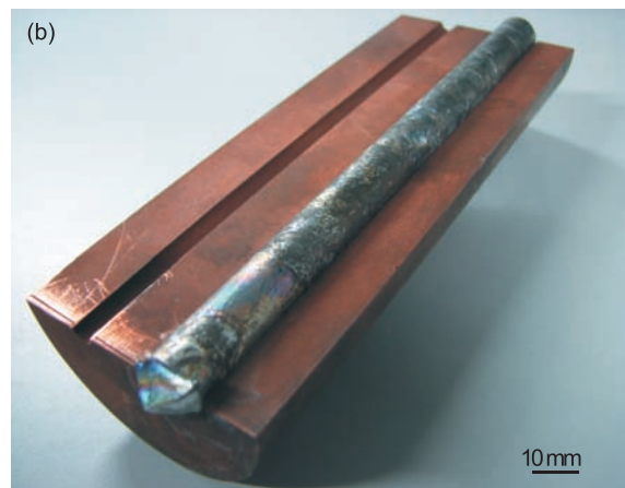
Fig. 8: Sketch map of copper mould (a) and its casting (b)
