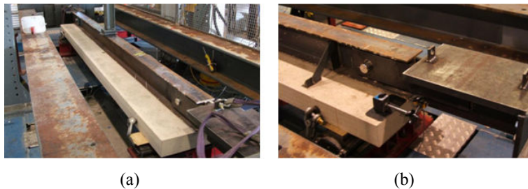
Fig. 1. (a) Test set up for Negative Bending and Axial Tensile loads (b) Load Applicator to Axial Tensile Loads [2].
