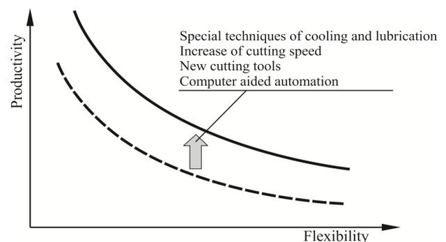
**Fig. 1.** Possibilities to increase the productivity of manufacturing.
