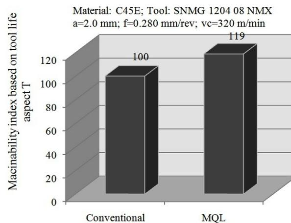
Fig. 27. Values of machinability index based on the tool life aspect.
