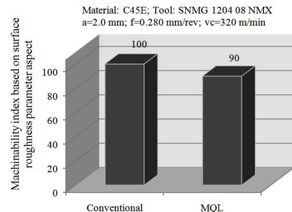
Fig. 28. Values of machinability index based on surface roughness aspect.
