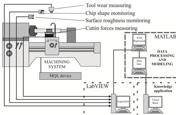
Fig. 8. Data flow in measuring and monitoring.
