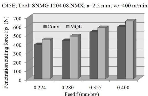
Fig. 11. Values of penetration cutting force.
