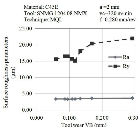
**Fig. 16.** Changes of parameters  $R_a$  and  $R_y$ , depending on the tool wear in machining with MQL technique.
