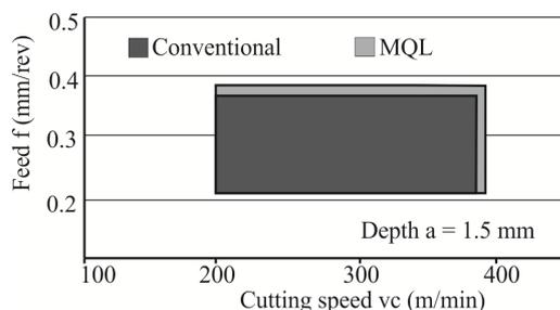
**Fig. 12.** Technological areas for depth  $a = 1.5$  mm.
