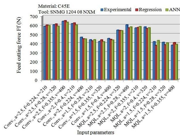
Fig. 21. Output values of the feed cutting force from regression model and ANN model.
