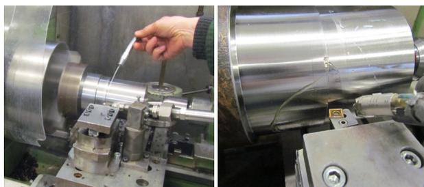
Fig. 6. Position of conventional flooding (left) and MQL nozzle (right) during the experiments.
