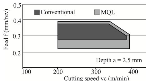
**Fig. 13.** Technological areas for depth  $a = 2.5$  mm.
