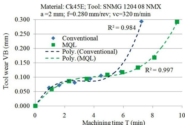
Fig. 23. Modelled curves of tool wear for different lubrication technique in machining steel C45E.
