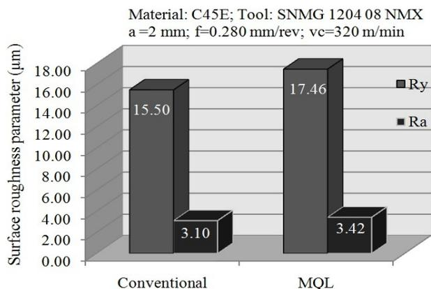
Fig. 18. Values of surface roughness parameters for different lubrication techniques.
