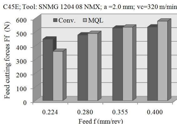
Fig. 10. Values of feed cutting forces.
