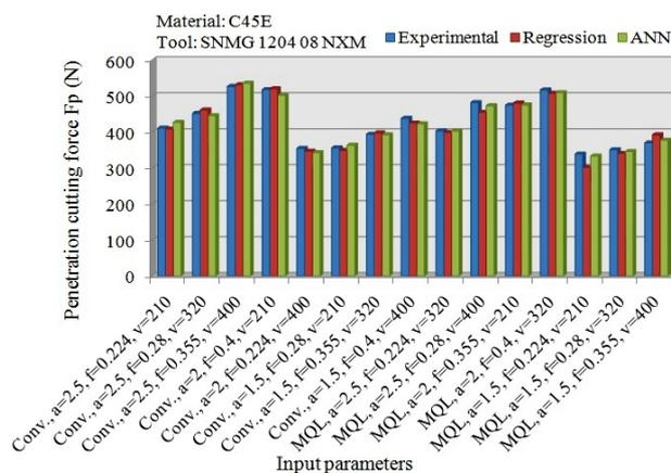
Fig. 22. Output values of the penetration cutting force from regression model and ANN model.
