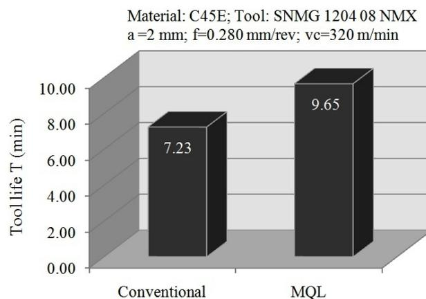
**Fig. 17.** Values of tool life for different lubrication techniques.
