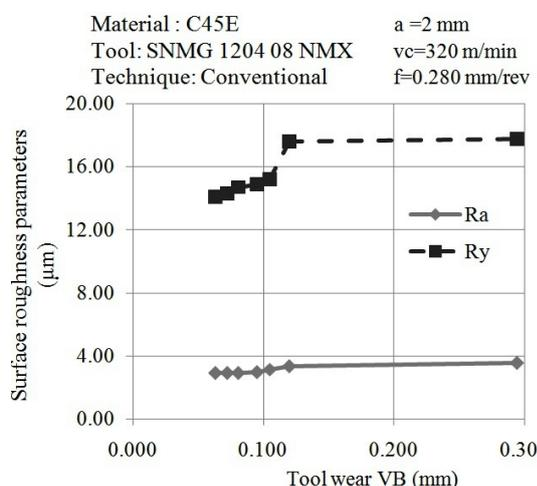
**Fig. 15.** Surface roughness regarding the tool wear in machining with conventional CLF dosing.
