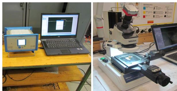
Fig. 7. Measuring devices: force data acquisition (left) and tool microscope (right)
