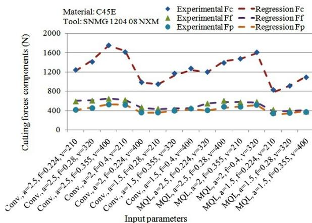
Fig. 19. Comparison of outputs regression model with experimental results.
