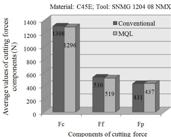
Fig. 9. Comparison of the mean value of components of cutting force for both dosing techniques.
