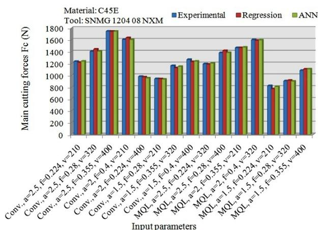
Fig. 20. Output values of the main cutting force from regression model and ANN model.
