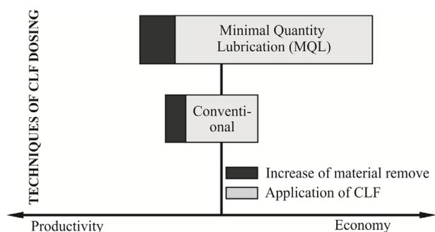
Fig. 3. Influence technique of lubrication on productivity and efficiency.
