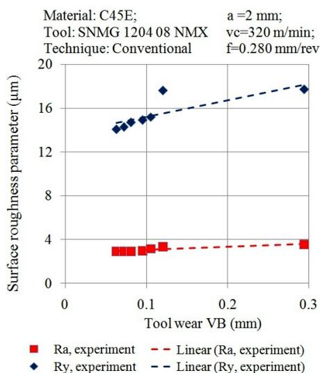
Fig. 24. Models of parameters roughness for the conventional technique of CLF dosing.
