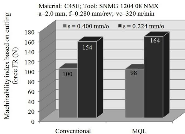
Fig. 26. Values of machinability index based on energy aspect.
