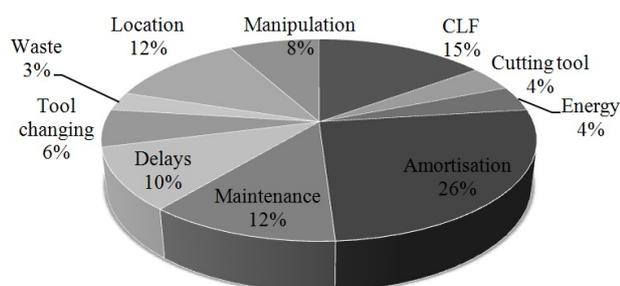
Fig. 2. Structure of the machining costs.
