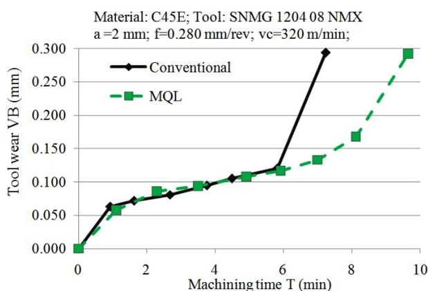
**Fig. 14.** Comparative diagram of tool wear for different techniques of CLF dosing.
