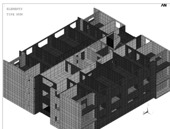
Fig. 4. Model of the panel building – detail.
