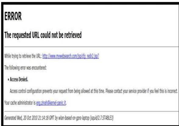
Fig. 10. Client's Request out of Allowable Time was Rejected.
