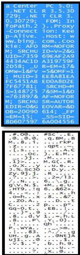
Fig. 12. Plain and Encrypted Packets within the SSH Tunnel.
