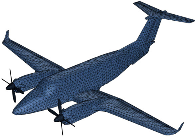
Fig. 1. Discretisation of the platform model with 15 680 triangles for analysis up to 118 MHz.
