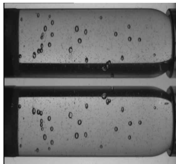
Figure 5. The image of the bubble detector taken by the automatic bubble reader after the exposure to neutron operated with the deuteriated titanium target
