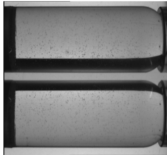
Figure 3. The image of the bubble detector taken by the automatic bubble reader before the exposure to neutron
