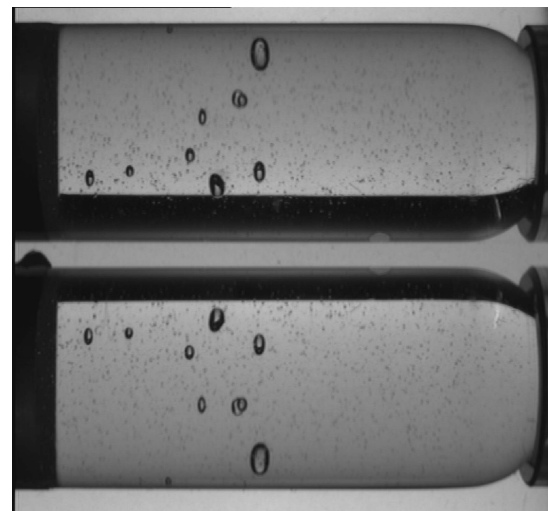
Figure 4. The image of the bubble detector taken by the automatic bubble reader after the exposure to neutron operated with the drive in titanium target
