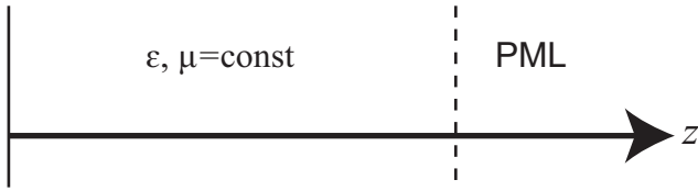
Fig. 3. Test structure with perfectly matched layers
