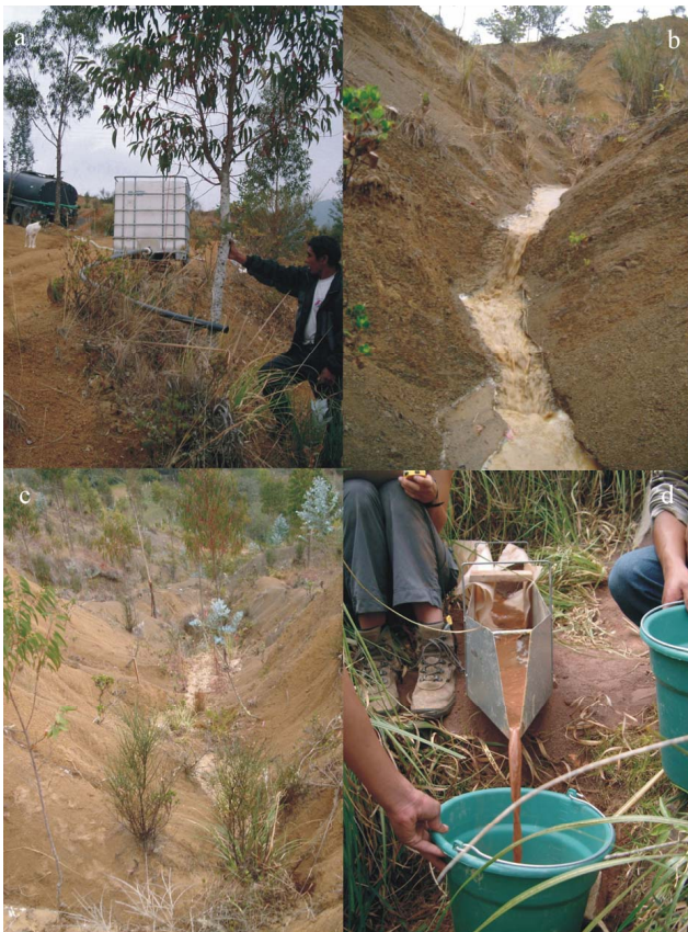
Fig. 2. Experimental design of the concentrated flow experiments with (a) water supply from water tank, (b) and (c) concentrated flow in the gully floor, and (d) collection of runoff water and sediment.
