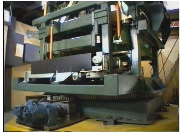
Fig. 3 .TEM six-component balance
