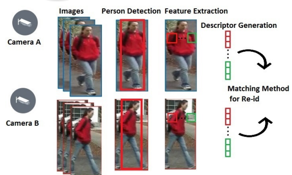
Figure 1: In person re-identification multiple images of a person are collected by camera A and B. Person detection algorithms are applied on captured images to separate person from background. Then features are extracted from images to represent a person. All the extracted features are concatenated to generate a descriptor. Then descriptors matching is performed for identification.
