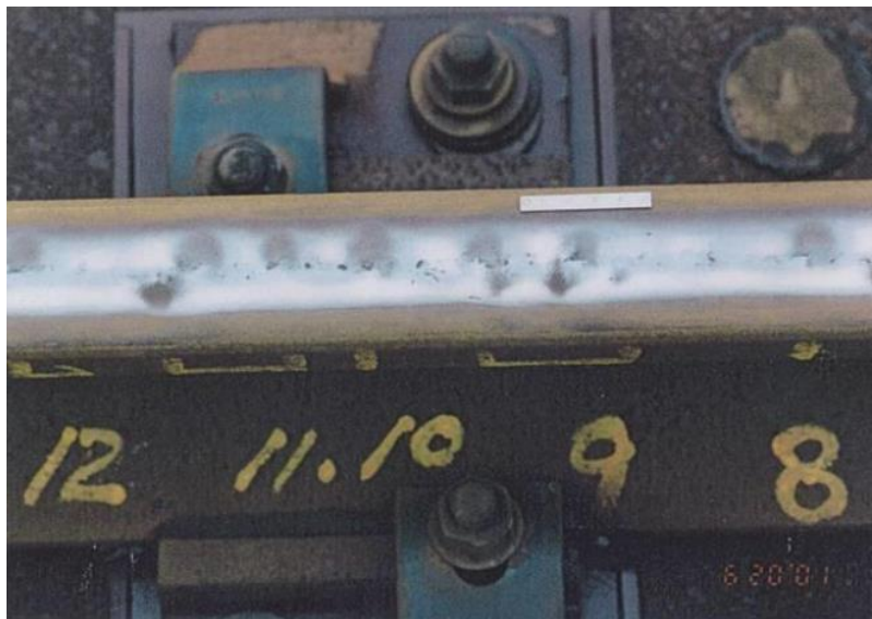
Figure 2: Multiple short-pitch rail surface defects.
