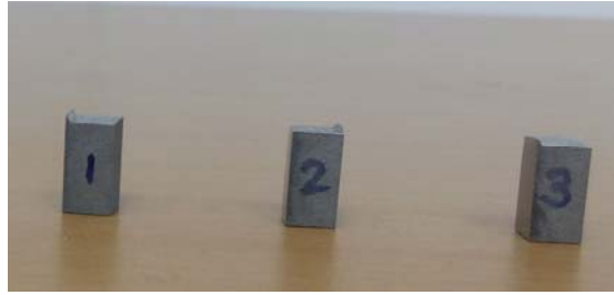
Fig 9. SLM coupons fabricated using the optimized process parameters
