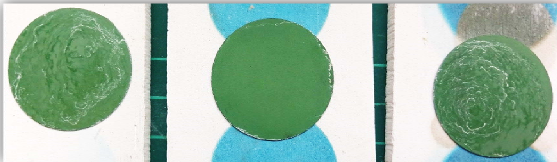
Figure 7: Cells doped with AMT in water with pre-wet spray showing inconsistent ring-like patterns.
