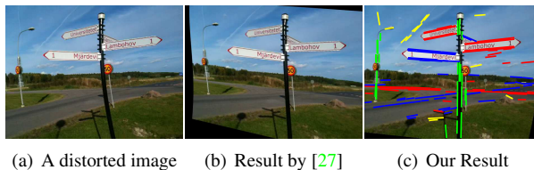
Figure 1: (a) A real rolling shutter distorted image. (b) Rectified by Rengarajan et al. [27]. (c) Proposed joint estimation of orthogonal vanishing directions and rolling shutter motion. The colors red , green and blue are employed for the orthogonal vanishing directions, while yellow is used to mark the outliers (lines that are not associated with the vanishing directions). Sign-post and roads are more geometrically consistent by the proposed method.
