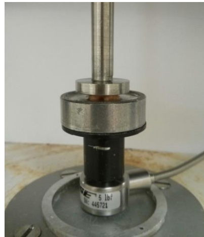
Figure 2 – Compressive DMA set-up for human bladder tumours.
