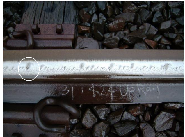
a) High rail typical of squat features in a squat zone
