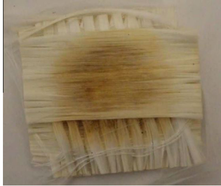
Fig. 3. Evidence of diffusion limitation on a 50 × 50 mm GFRC sample after hydrolysis in a 20 L reactor (temperature assumed to be around 300 °C according to the report) [113].
