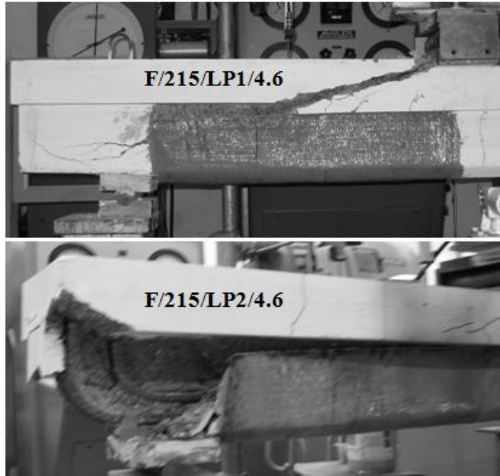
Fig. 7–F/215/LP1/4.6 and F/215/LP2/4.6 at failure.
