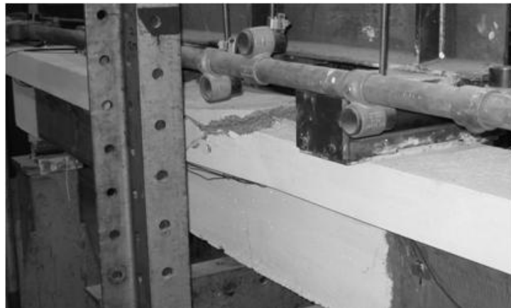
Fig. 8–Flexural failure of F/295/LP1/3.3.
