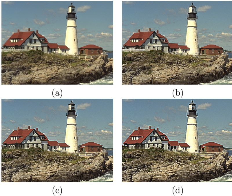
Figure 3.4: Effects of increasing window size in AEBCE technique (a) original image [b-d] enhanced image with different window size (b) 3 \times 3 (c) 5 \times 5 (d) 7 \times 7
