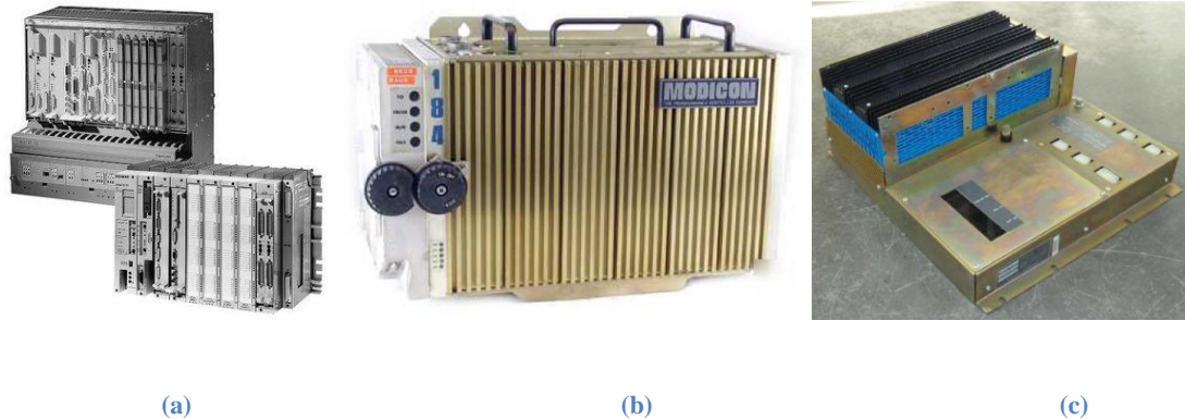
Figure 10 - Modicon 084 & 184 and Allen-Bradley 1774 PLCs
