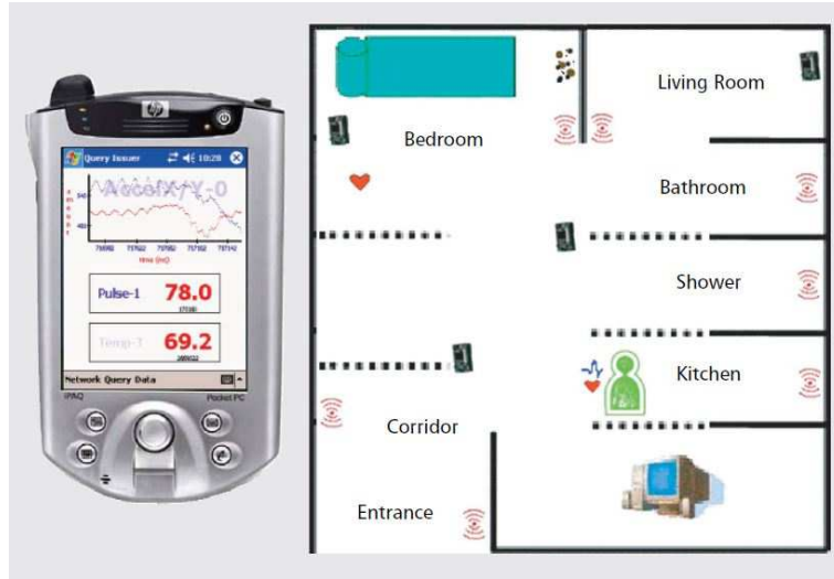
Figure 3.3: PDA AlarmNet[12] administration GUI and system architecture.
