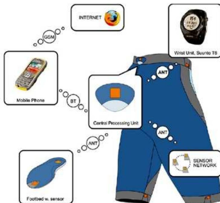
Figure 2.3: HipGuard: a garment integrated measurement system [3].
