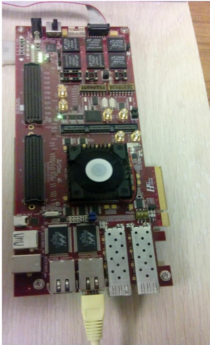
Figure 33: Virtex 6 XC6VLX550T FPGA Board
