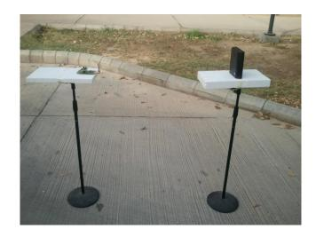
Figure 4.27 Measurement setup with 1 meter distance between the receiver and the transmitter
