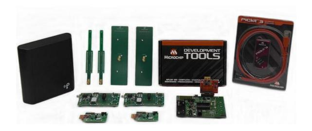
Figure 4.20 Powercast energy harvesting kit components [93]
