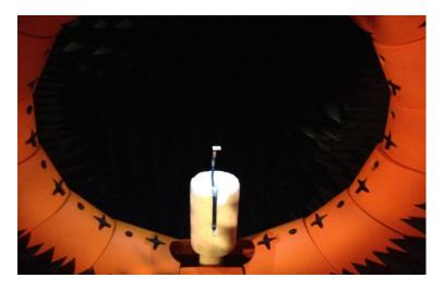
Figure 5.9 Patch antenna near field measurement setup
