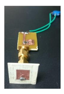
Figure 5.20 Fabricated 2.43 GHz rectenna
