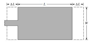
Figure 2.12 Patch antenna effective length [11]
