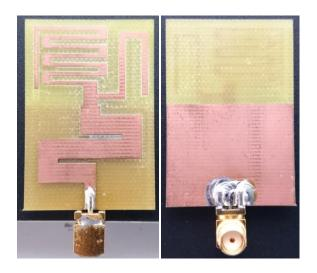
Figure 4.10 Fabricated MLA with  $\lambda/4$  transformer fabricated on FR4
