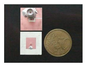
Figure 5.2 the fabricated patch antenna top and bottom layers
