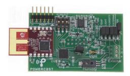
Figure 4.24 Wireless Sensor Board [93]
