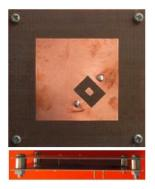
Figure 3.6 the fabricated dual polarized rectenna [25]
