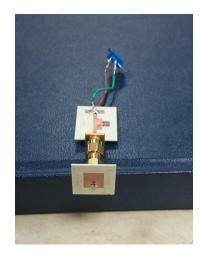
Figure 5.21 Fabricated 5.2 GHz rectenna
