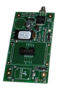
Figure 4.22 Powercast Evaluation Board (P2110-EVB) [95]
