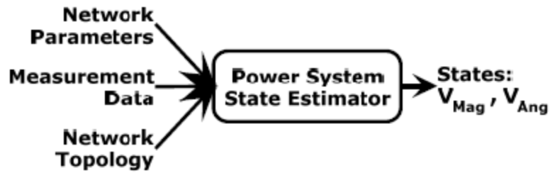
Figure 4-2 Input / Output of Power System State Estimator
