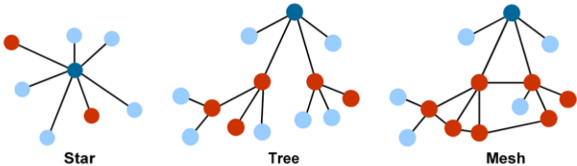
Figure 4-4: Various ZigBee Topologies
