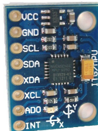
Figure 4.7: MPU6050 accelerometer + Gyro
