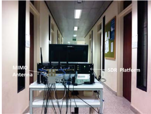
Figure 5.14: Measurement setup at the receiver end
