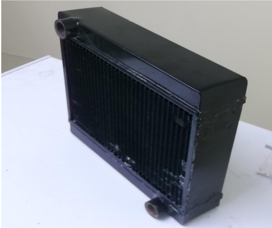
Figure A-2 Photograph of the pre-cooler for option 'A' before installation.
