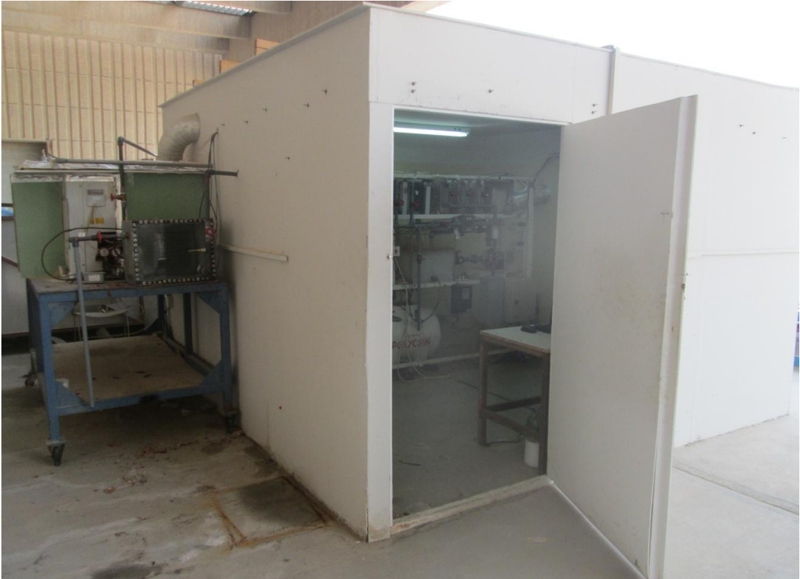
Figure A-11 Front-face of the completed experimental set-up showing the outdoor unit and subcooler.
