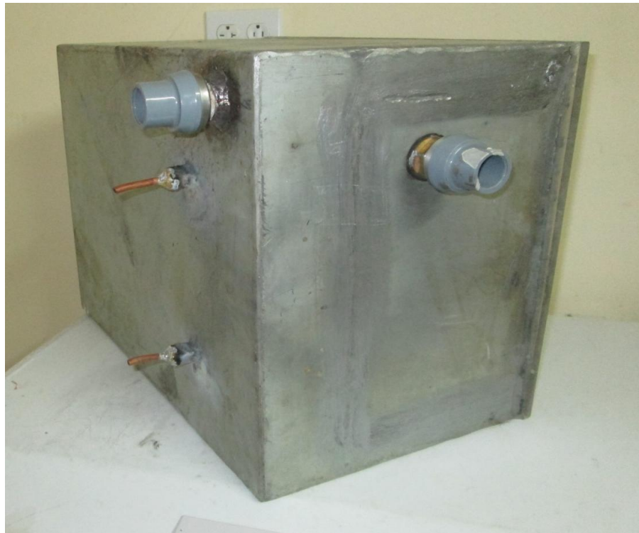
Figure A-9 Three-D picture of subcooler showing the refrigerant inlet and outlet connections.
