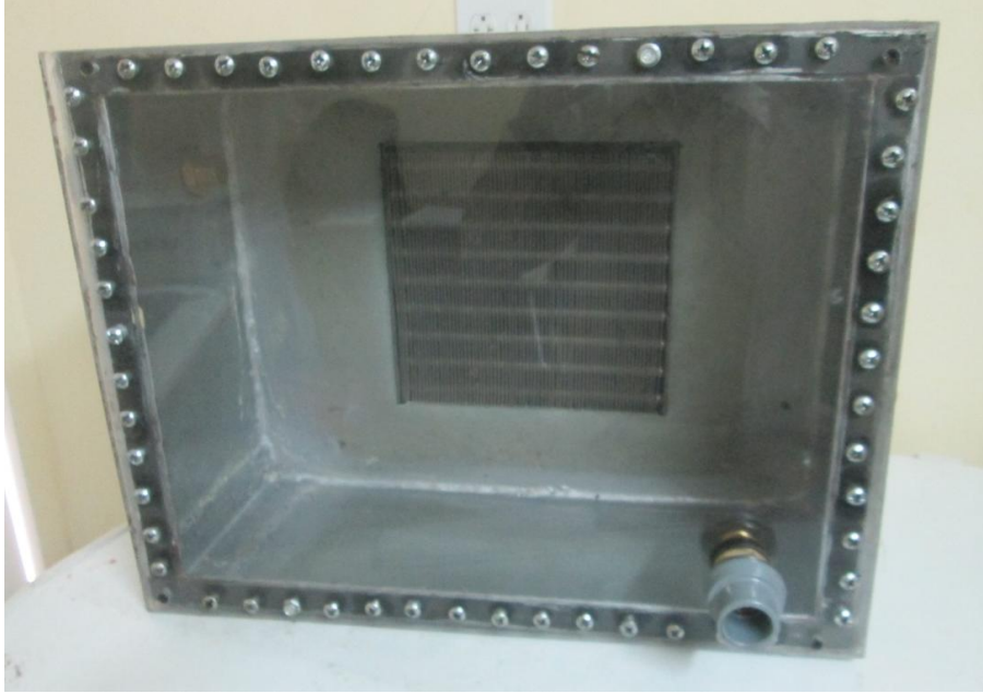
Figure A-8 Glassed-face picture of subcooler showing water inlet before installation.
