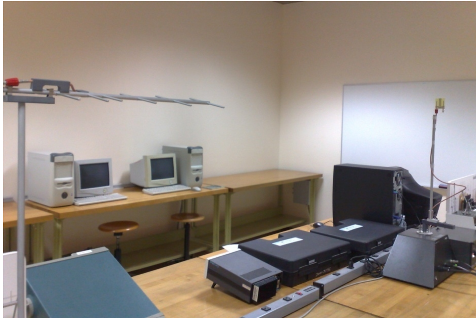
Figure 5-14 Experimental Setup for measuring the gain/radiation pattern
