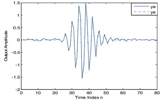
Figure 3: Actual & estimated output signals at 5 dB SNR
