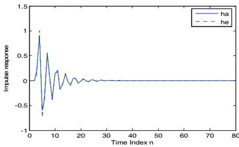
Figure 2: Actual and estimated IR signals at 5dB SNR
