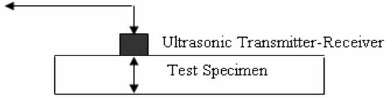
Figure 1: Pulse Echo Flaw Detector
