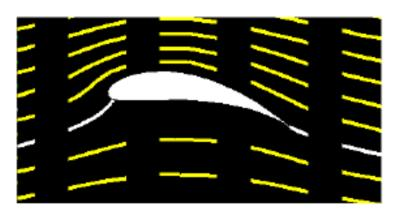
Flow turning at trailing edge is very important.
