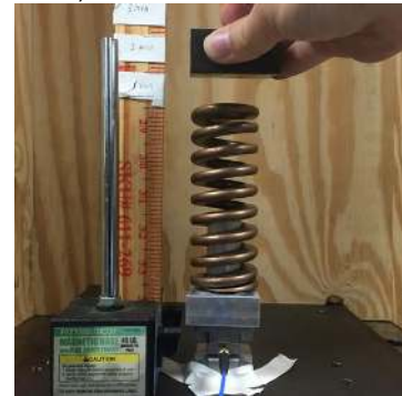
Figure 7 Impact force calibration test
