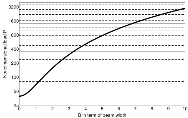
Fig. 4 The non-dimensional load as the function of the observed mid-span deflection (solid line); the mid-span deflection is traced in the units of beam width. The thin and the dashed horizontal lines represent the critical loads for two families of solutions w_{s_2}^n(x) and w_{s_3}^k(x) respectively.
