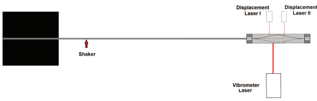
Fig. 13 The scheme of the experimental setup for the measurements with a steel beam as a primary system.
