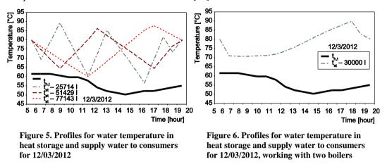
In the case of higher outdoor temperature, which is the case in 50% of heating season, the solution with 2 boilers is more acceptable. Only one boiler would be in operation, with short periods when the boiler is turned off. Figure 6 shows temperature profiles for heat storage volume of 0.05 m<sup>3</sup>/kW for March 12 with two 300 kW boilers. The boiler was in operation for the larger part of the day. Besides covering the heating demand, heat storage was charged as well.
