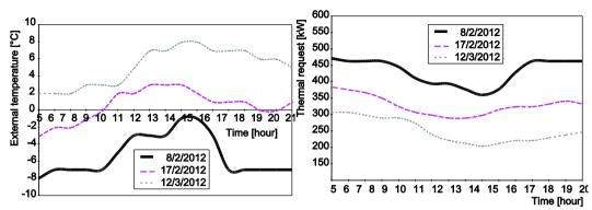
Figure. 1. External temperature variation with time of reference days
