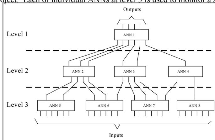
**Figure 3. Hierarchical Structured Artificial Neural Network**
