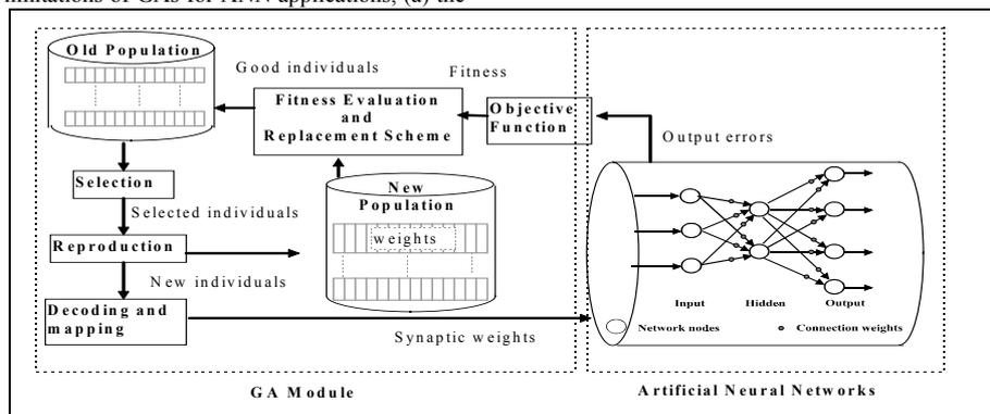
Figure 2. Block diagram of GA training method.
