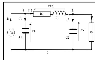
Figure 4. The schematic diagram of the  $\Pi$  circuit.
