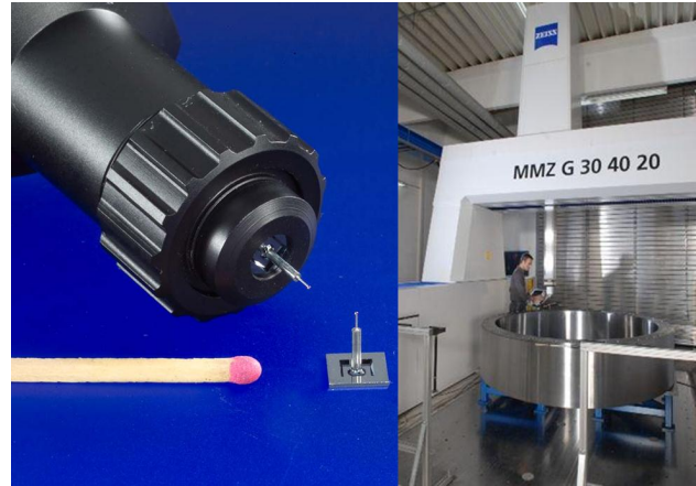
Figure 6. Accuracy in coordinate metrology in micro-scale, e.g. probe of a micro-scale part measuring device (Wiedmann et al., 2011), and macro-scale parts, e.g. measurement of large mechanical parts for wind energy systems (DeGlee, 2010).
