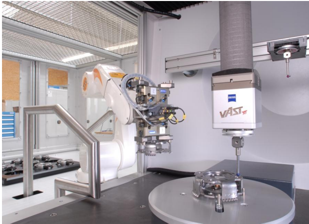
Figure 5. Faster metrology due to the automated integration of metrology into material flow with the aid of a robot.
