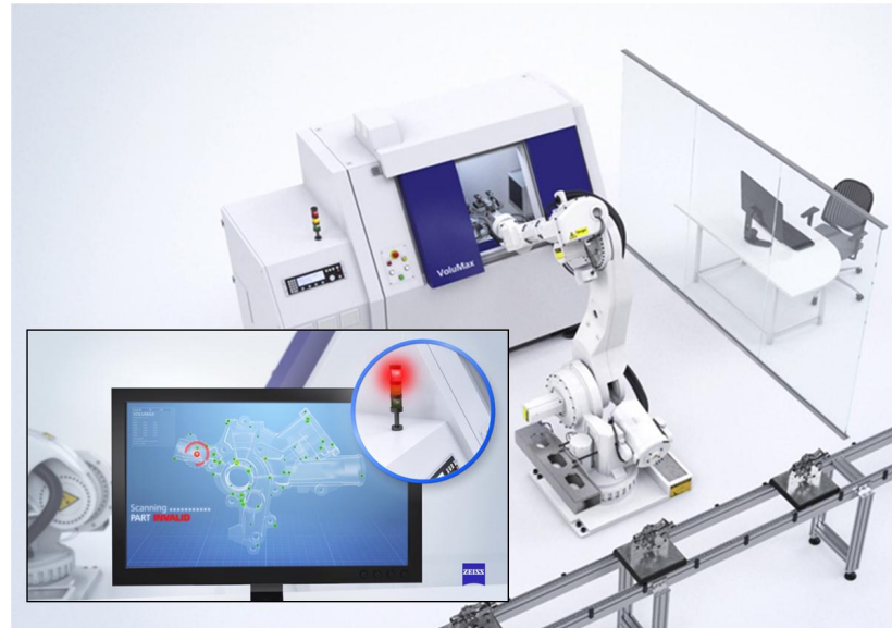
Figure 9. Computer tomography system for defect detection for in-line service.
