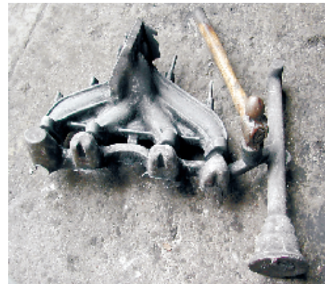
Fig. 4(b) A photo of the casting tree, showing the top filling gating system
