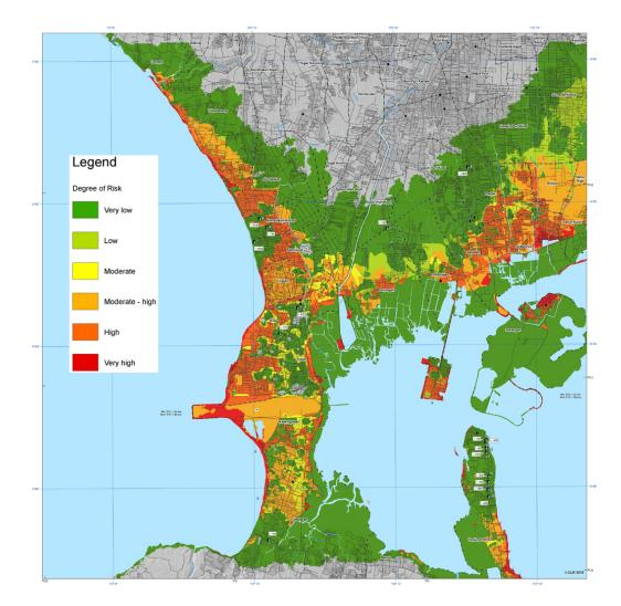
Fig. 13. Risk map of Kuta (Bali) highlighting the areas (in red) with high needs for tsunami evacuation buildings.
