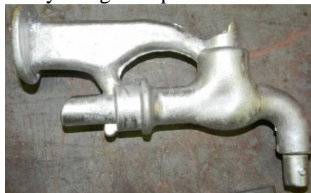
Fig. 1. A part obtained through casting used for experiments
