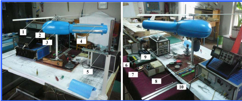
Fig.7 Experimental device: 1-NOTAR helicopter blades carbon fiber, 2 -hub pitch, 3-structure helicopter fiberglass,
