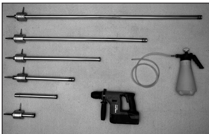
Fig. 1. Selection of 25 mm diameter drill-core bits (up to 1.3 m in length) used to core flowstone and tall stalagmites together with the drilling machine and the water supply system. On the second smallest drill-core bit the SDS adapter and the water flushing system were removed.
