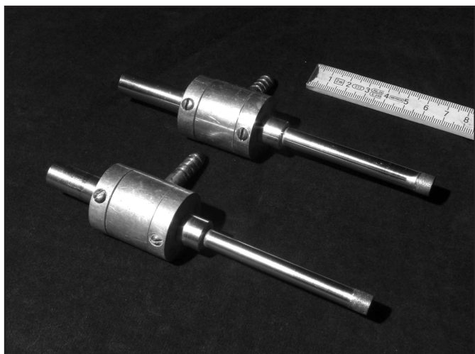
Fig. 4. Two small-diameter drilling bits (cm-scale) used to obtain cores samples (5.6-6.9 mm diameter) for reconnaissance dating of in-situ stalagmites.
