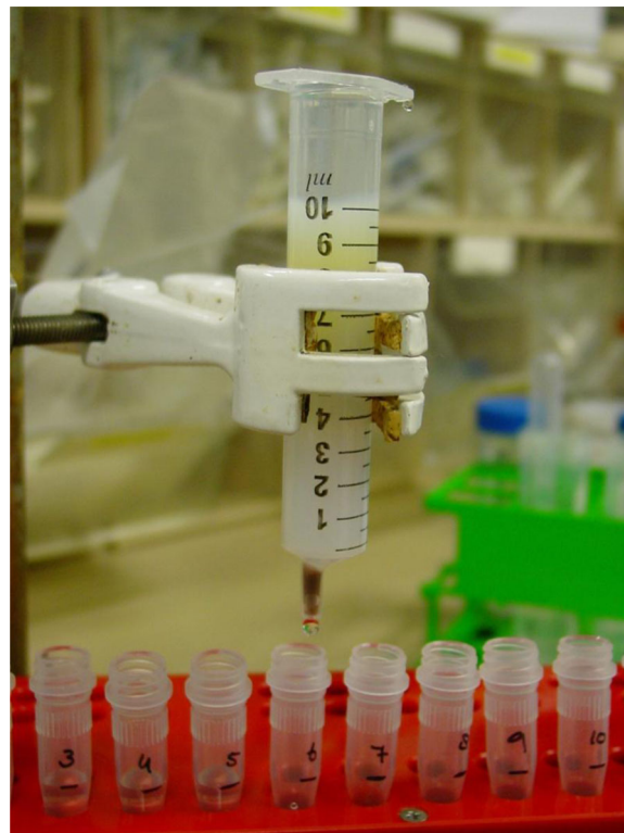
Fig. 1. Image of size-exclusion chromatography column. A 10 mL syringe stacked with sepharose CL-2B for isolation of vesicles from platelet-free supernatant of platelet concentrates.
