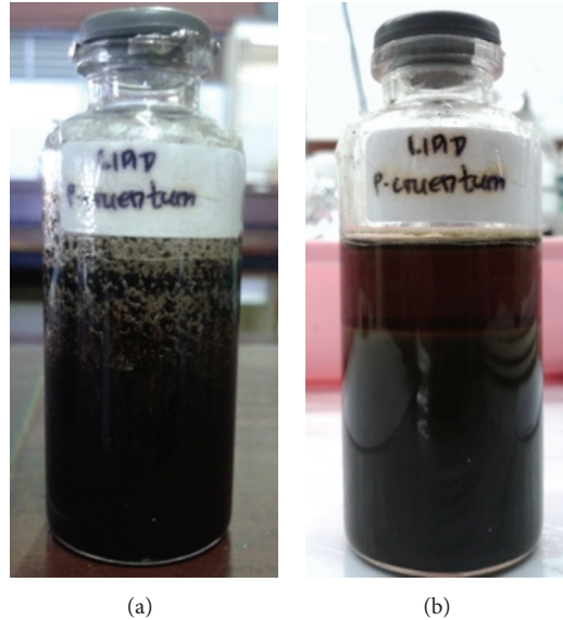
FIGURE 2: (a) Lipid of phytoplankton Porphyridium cruentum . (b) Result of transesterification reaction.
