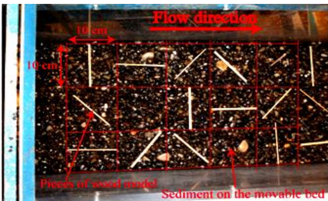
Figure 8. Initial situation of wood pieces on the movable bed in the flume.
