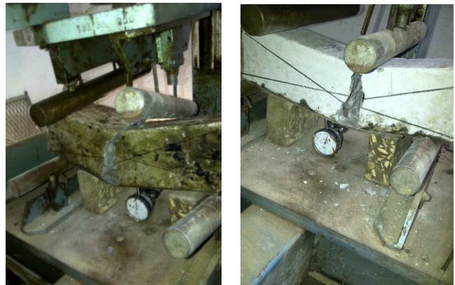
Figure 12. specimen beam pattern collapse
