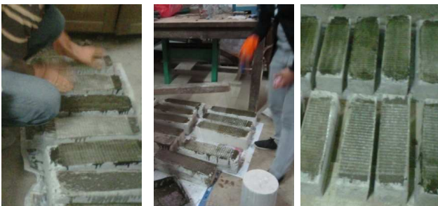
Fig. 3. Installation of GFRP Sheet on the beam
