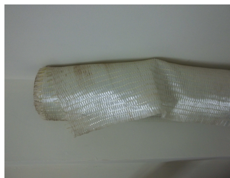
Fig. 1. Glass fiber sheet
