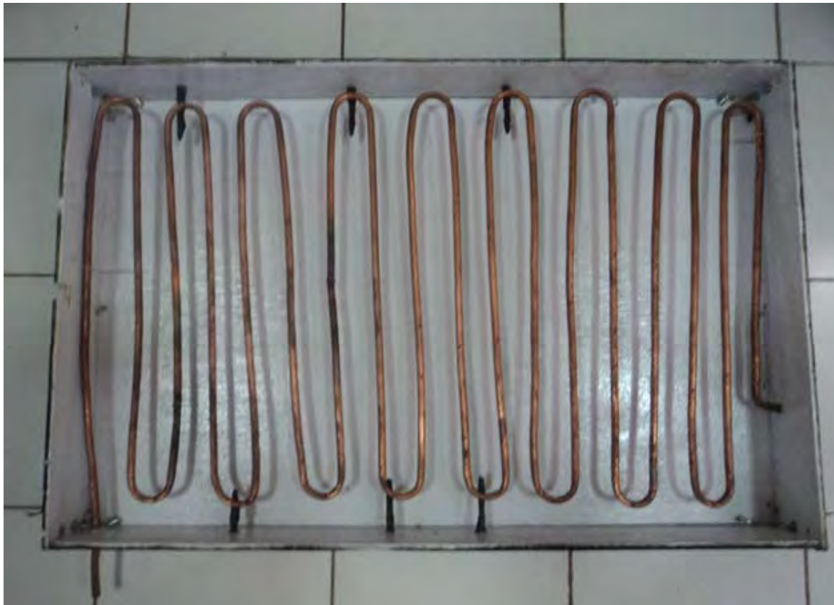
Fig. 1. Construction of spiral Copper pipe in the box extraction
