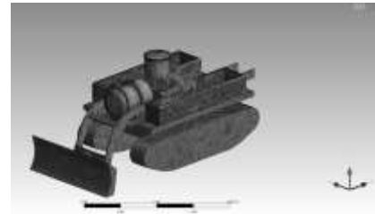
(c) Structural mesh
